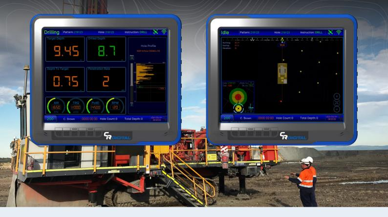
Thunderbird 1110 is a high-precision GPS and rock strata measurement system for rotary blast drills. Paired with CR Digital's Orion Data Analytics, Thunderbird 1110 provides drill & blast managers unsurpassed insights on drilling performance through unique cloud-based data analytics.
